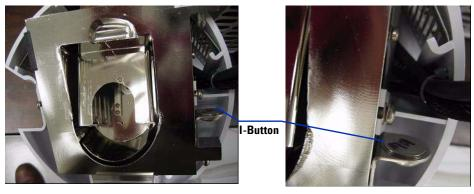
Figure 16 Multimode source with I-Button
